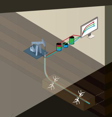
Pipe-It Shale Solution uses daily production data from horizontal multi-fractured wells to numerically model reservoir, fracture and well characteristics. This provides more accurate predictions of future well performance under different production conditions, including uncertainty analysis.
