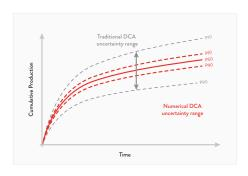
Generate reliable decline curves for a section / area based on the detailed single well analysis.
